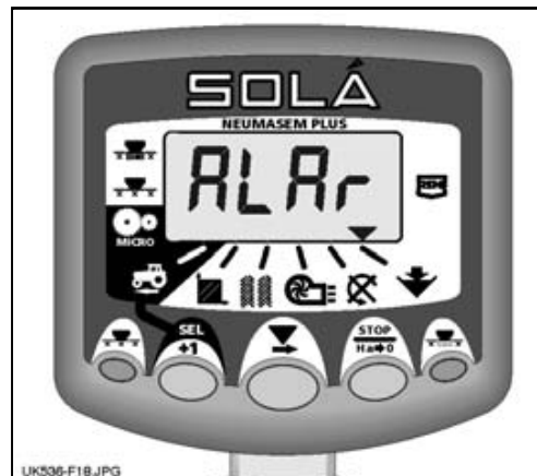
Figure 18: Hopper Low Alarm
